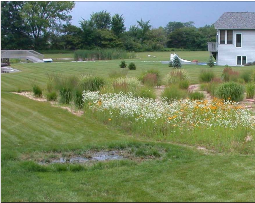
Figure 2. Septic system failure due to hydraulic overload. The soil absorption field could not accept the volume of water discharged from the home, resulting in septic tank effluent coming up to the ground surface.
